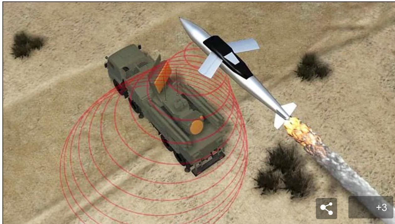
**Graphic shows the Counter-electronics High Power Microwave Advanced Missile Project (CHAMP) missile taking out a target. In a test in the Utah desert, the missile successfully defeated electronic targets with little to no collateral damage**
